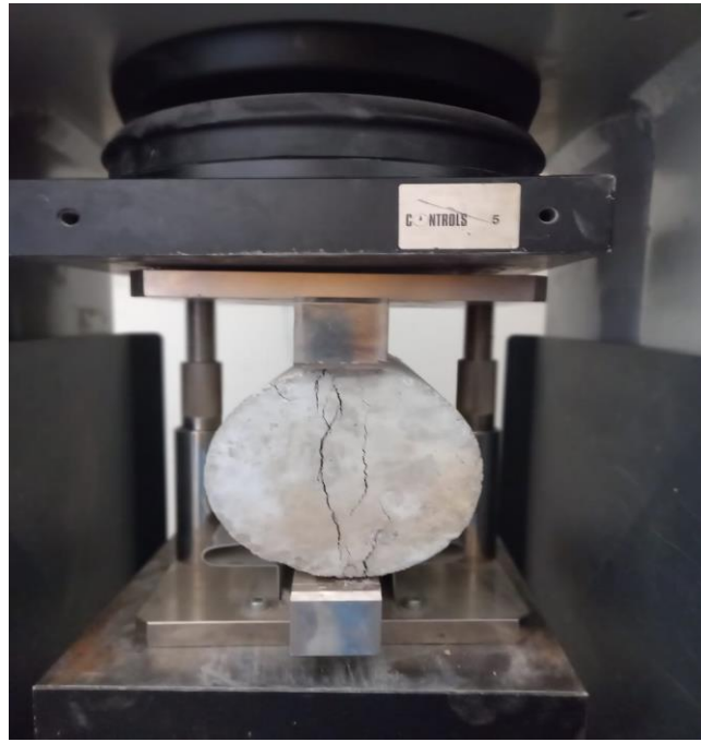
Figure 4: Split Tensile test on Partially Replaced Concrete.
