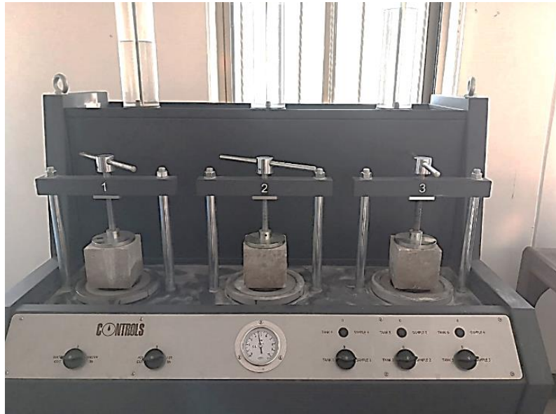
Figure 6: Cubical Moulds in Water Permeability Apparatus
