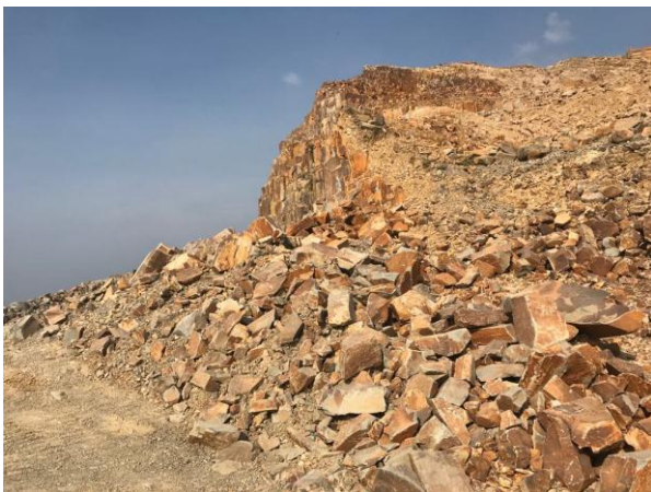
Figure 3: Jointed weathered rock at upper section of the hill (~RL170).
